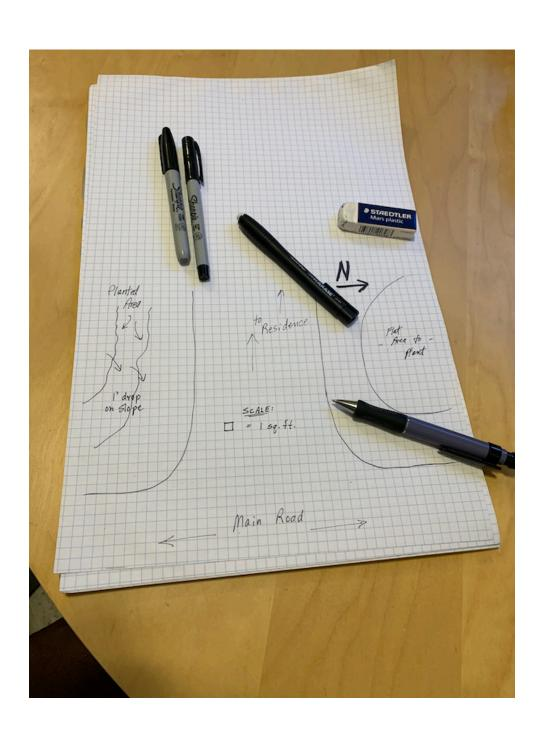
Standard private road width for rural properties is 15' across (12' is the absolute minimum for emergency vehicles.) Next up - drainage. You'll want a gentle slope off either side to allow moisture to runoff & snow to drift over the driveway surface (think of how a highway ditch allows snow & rain to drain from the pavement)
